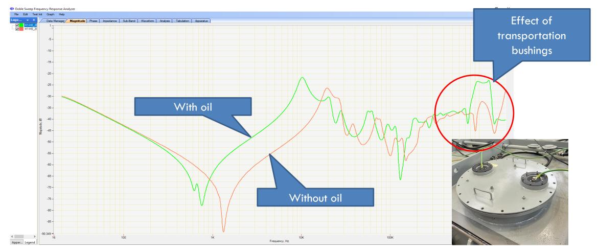
Measurement in fully assembled condition and in transportation condition
