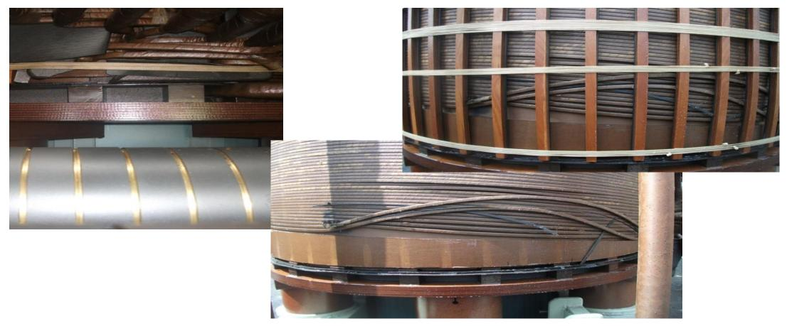
Luckily it was possible to see damage through inspection hole. Scrapping confirmed slight winding deformation on A phase
