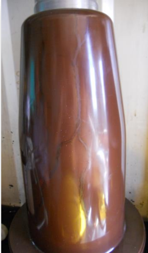
White phase GIS termination disassembled
