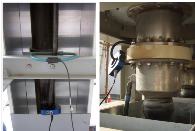
Sensors connection at terminations
